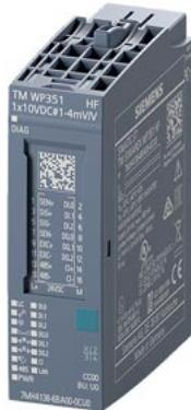
SIMATIC ET 200SP, TM SIWAREX WP351 HF, single-channel calibratable weighing module for automatic dosing-, filling-, checking- and totalizing scales with analog load cells, 3xDI, 3xDQ, 1xCI, 1xRS485, 1xEthernet, 1xLC load cell interface (1-4mV/V), suitable for BU type U0, packing quantity: 1 unit
